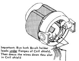
Field and Brush Holder Wires Should be tied Together with Wire Tie 23-78-0100
